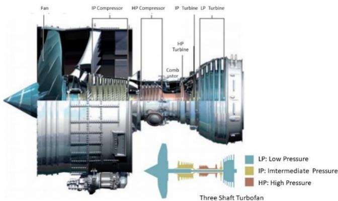
Figure 2 – Layout of a turbofan (courtesy Rolls-Royce)
